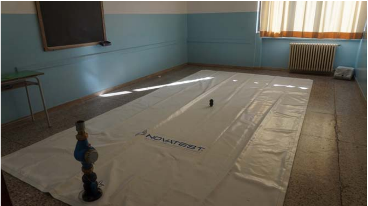
serbatoio in PVC
